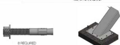
FOOT PLATE TO FLOOR CONCRETE CONNECTION DETAIL
